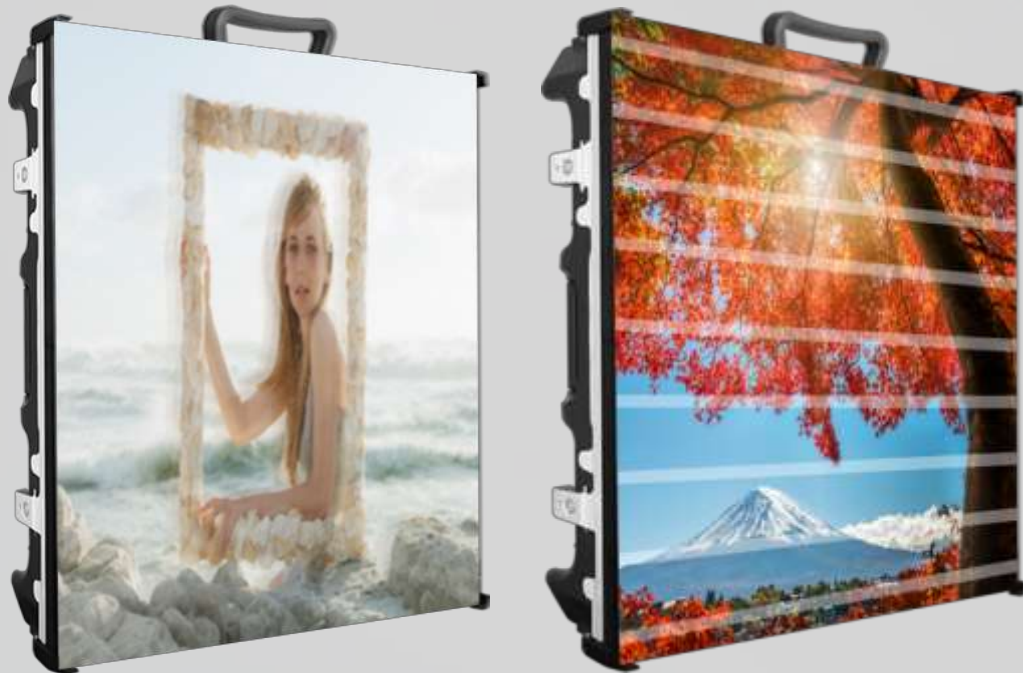
▲ Display defects on low refresh rate LED cabinets
