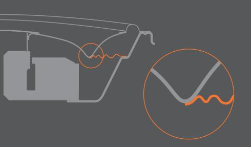
Secondly, rather than attaching the suspension conventionally to the voice-coil former, it attaches to the diaphragm at the point where its profile changes from curved to dome. This change of suspension mounting location enables the motor system to be brought much closer to the underside of the diaphragm and so reduce again the depth of the complete assembly.
