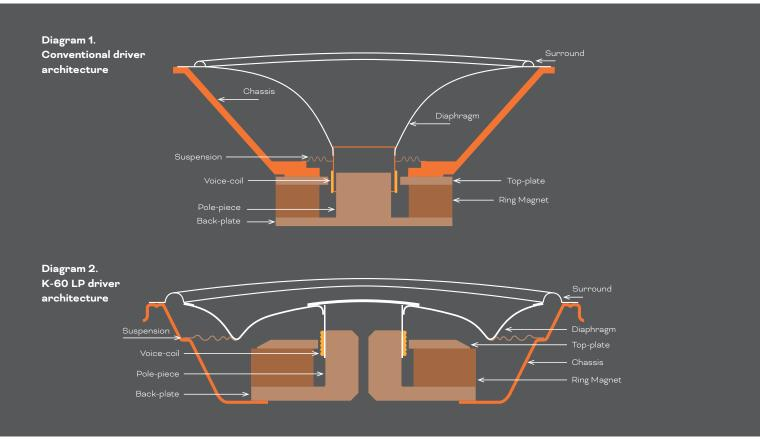
Firstly, the curved outer region of the diaphragm joins a large convex domed region towards its centre. The combination of a curved outer region and a central domed region provides structural rigidity equivalent to that of a conventional diaphragm, however it also offers much reduced overall depth.
